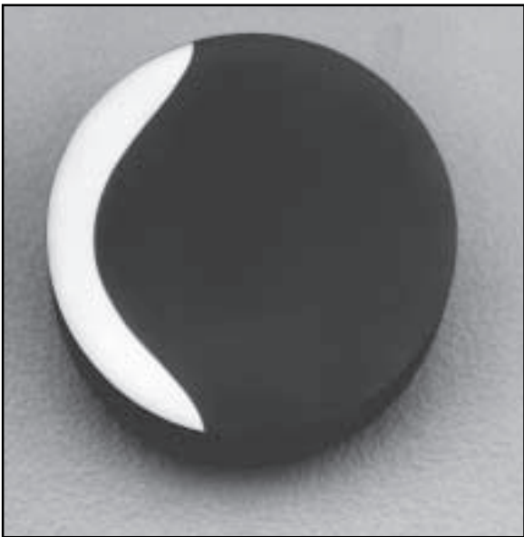
A cross section of a selectively induction hardened WHX pin – the crescent area is super-hardened to dramatically lengthen pin wear life. The balance of the pin material is left in the thru-hardened condition to give the pin excellent toughness.
